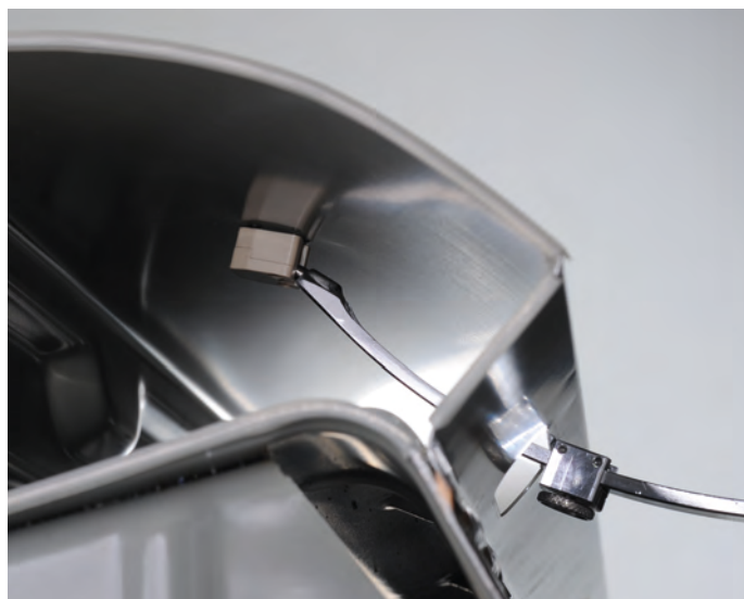
Car body in section to show how the probe V3FGA06H measures the EPD coating within the car body.
