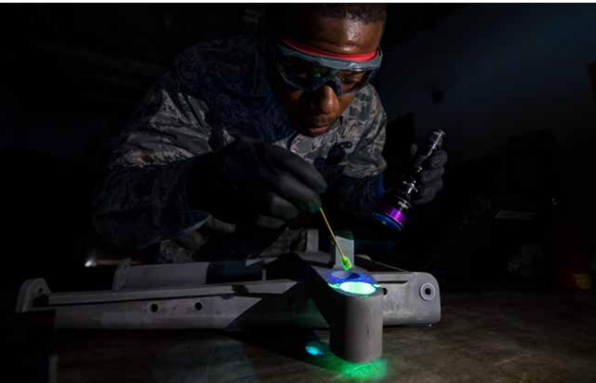
NDI Technician of the 5th Maintenance Squadron is testing for cracks and imperfections on B-52H Stratofortress parts and aircraft support equipment with a UVG3 UV light at Minot Air Force Base, N.D., Jan. 25, 2019.
