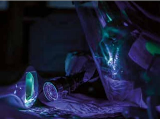
NDI Technician of the 5th Maintenance Squadron non-destructive inspection journeyman, shines a Labino UVG3 UV light during a fluorescent penetrant inspection at Minot Air Force Base, N.D., Oct. 18, 2016. The UV light helps locating cracks and imperfections on parts of the B-52H Stratofortress and aircraft support equipment.
