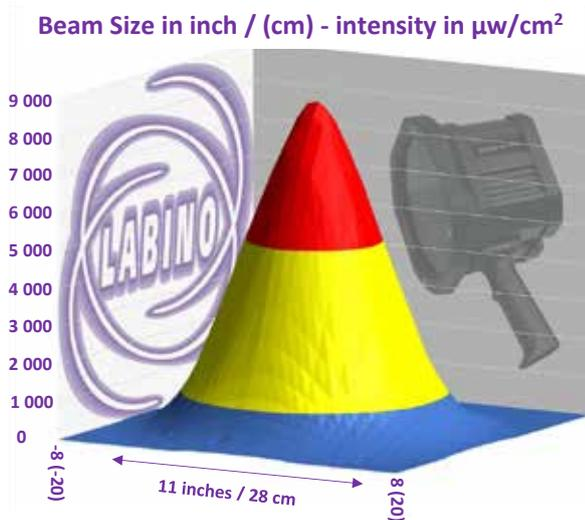
**Beam profile > 1 000  $\mu\text{W}/\text{cm}^2$  measured at 15 inches / 38 cm of BB 2.0 Artemis:**
