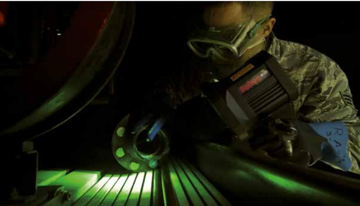
NDI Technician of the 108th Maintenance Squadron looks at cracks seen on a KC-135 Stratotanker part using a Labino BB 2.0 Series UV light, during a training session at Joint Base McGuire-Dix-Lakehurst, N.J., April 22, 2017.
