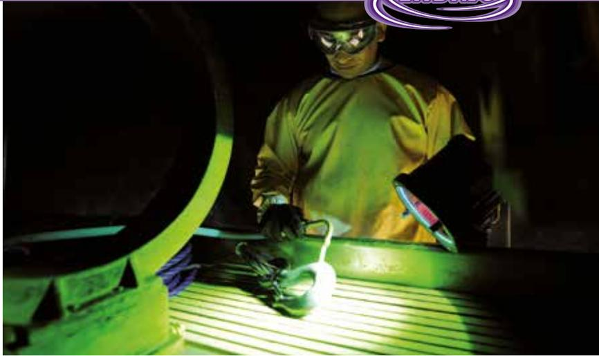
NDI Technician of the 28th Maintenance Squadron performs a magnetic particle inspection to search for any defects on a wire rope hook using a Labino 135 Series UV light at the Ellsworth Air Force Base, S.D.
