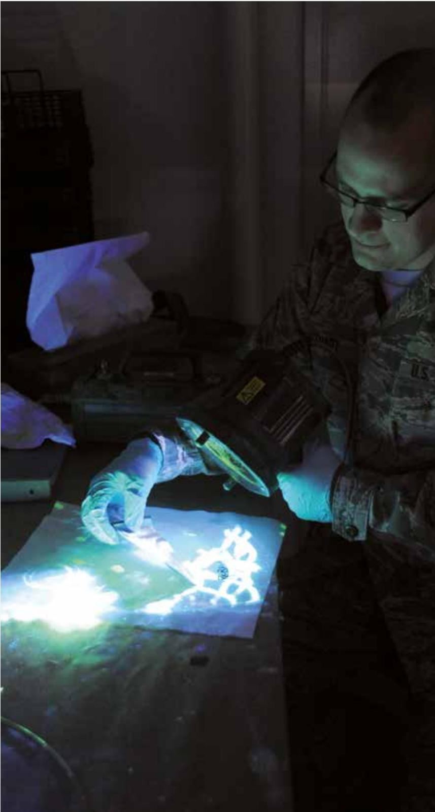
NDI Technician of the 180th Fighter Wing, uses a Labino BB 2.0 Series UV light to inspect an F-16 Fighting Falcon compressor blade for cracks during unit training assembly in Swanton, O.H.
