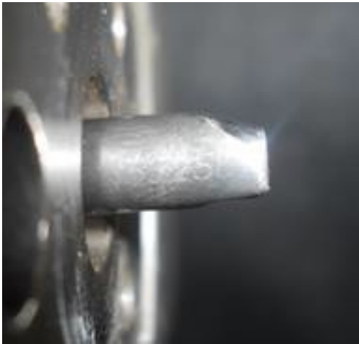
Excessively Worn Source Connector
