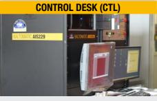
All elements are gathered in a control desk which can have different form and sizes. The control desk is feeding the system and hosting the necessary switches, fuses or breakers to make the installation as independent as possible. Most of our control desks are 19" compatible.
