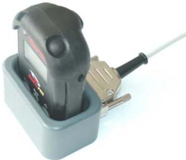
Communication between PC and SENTINEL RadEye G takes place via an optical adapter.
