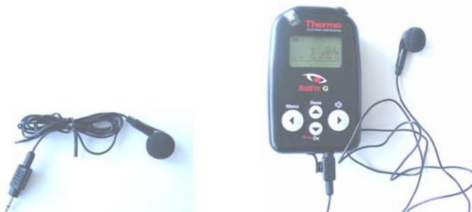
The earphone is connected at the bottom of the instrument after opening the rubber protection seal.
