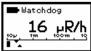
A Watchdog Error indicates, that the micro controller has problems to work on it's tasks in a given timeframe. Reasons are strong electromagnetic pulses, firmware errors or hardware issues.
