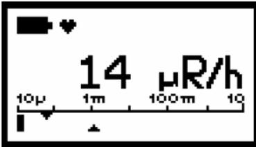
Typical display after switch on.
